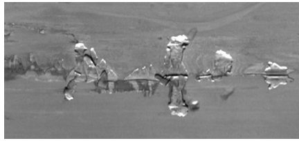
Lamination visualizations, highlighting defect areas of overlapping material of various shapes and sizes, irregularly distributed over the surface of the rolled material and often only partially bonded to the underlying surface.
